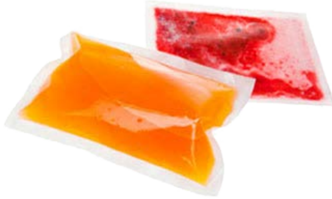
Figure 5.4. A single-use water purification device manufactured by Hydration Technology Innovations. The pouch is constructed with one side forward osmosis membrane and the other poly(ethylene). It is then filled with a sports drink powder and sealed. Water passes through the membrane, is purified, and then mixes with the drink mixture for consumption. Image courtesy of Hydration Technology Innovations and Eastman Chemical.
