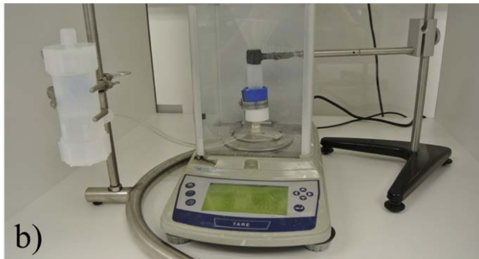
Figure 5.3. Schematic a) describing the apparatus used to perform real-time flux and water absorption measurements and b) image of the experimental setup.
